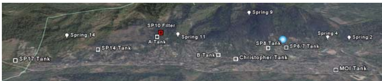
Figure 3-3: Major Water System Components.
